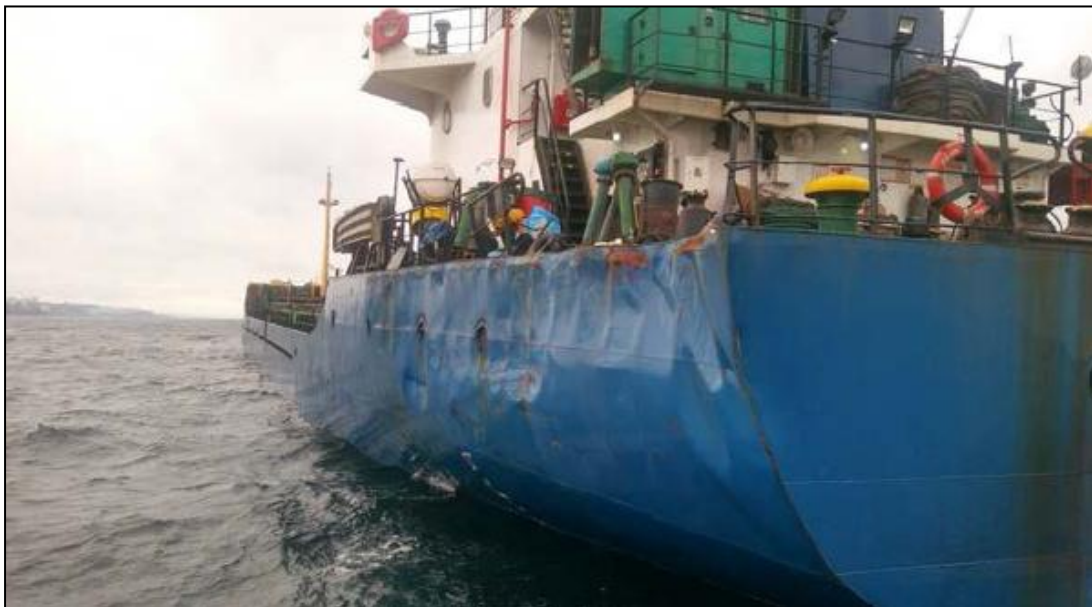
Figure 14: Damages in way of the poop deck and side shell plating
