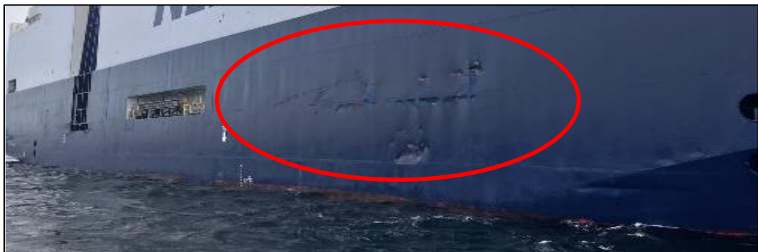
Figure 12: Damages in way of starboard side shell plating
