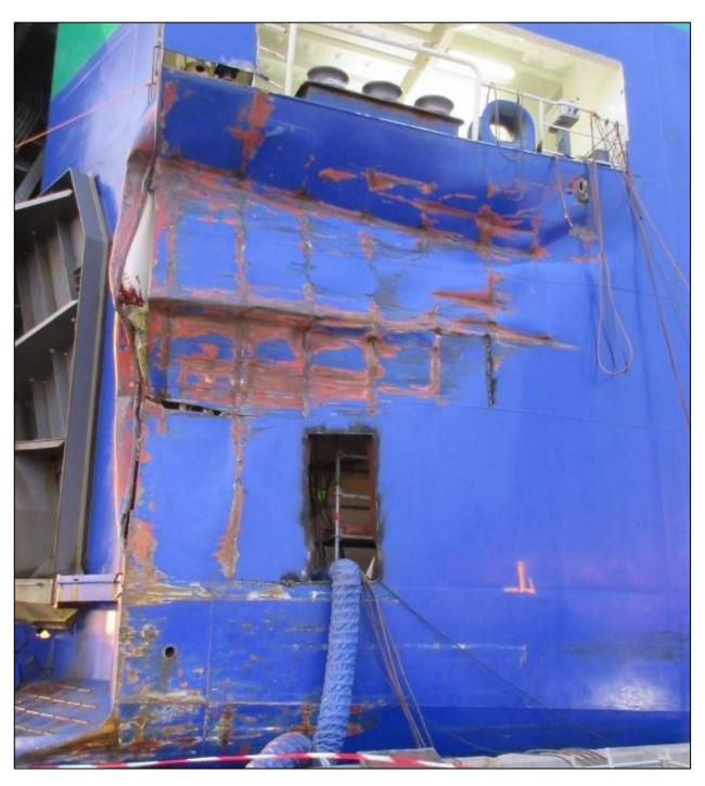
Figure 4: Ivory Arrow's damaged starboard transom
