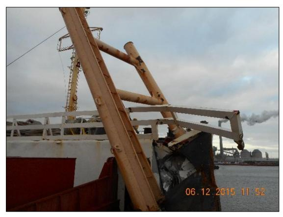
Figure 3b: View of damaged bulwark and log stanchion on Maraki
