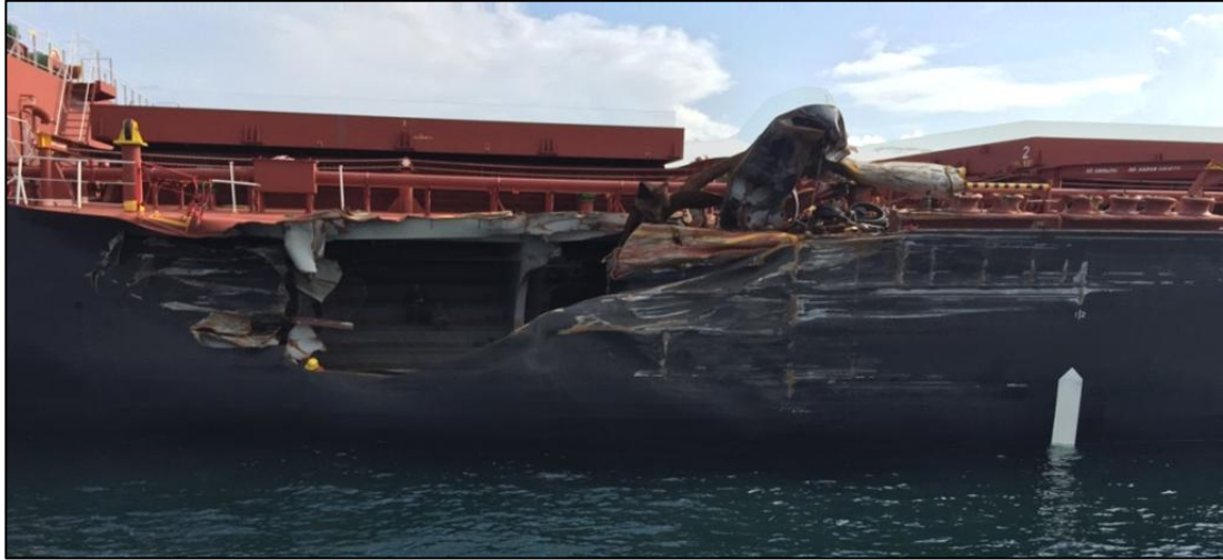
Figure 16: Point of contact and extreme damage section on Gortynia (port side)
