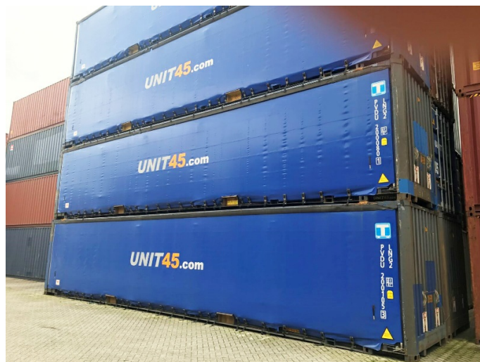
Figur 6.24 Open side container
