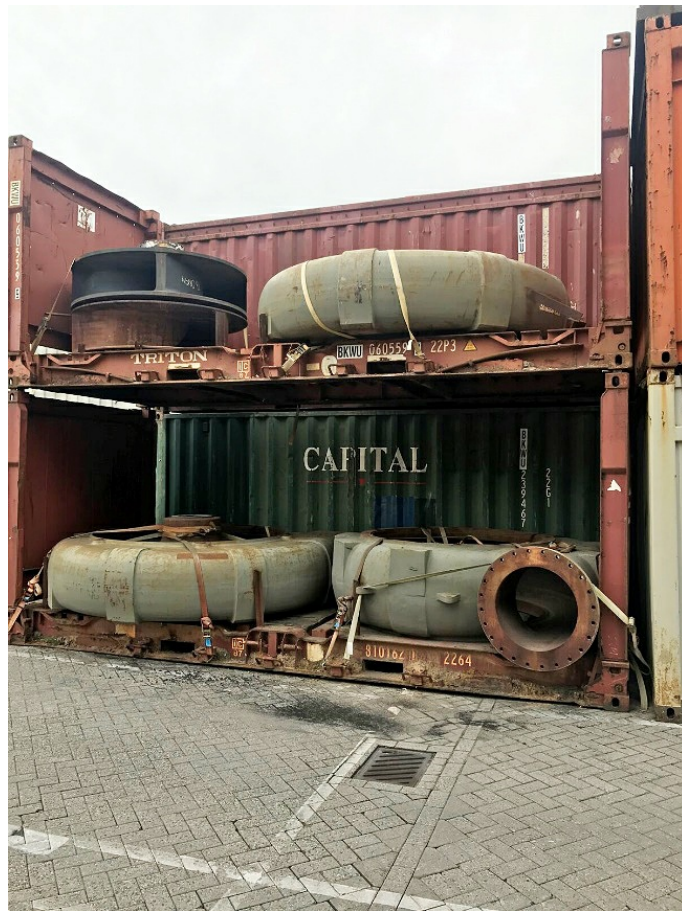
Figur 6.21 Flat rack container
